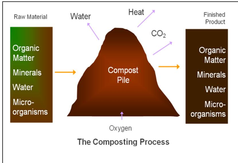
Human-controlled composting optimizes the conditions needed for the natural decomposition process. By creating these ideal conditions, a much faster and efficient decomposition of the organic waste and stabilization of the final product can be achieved.
