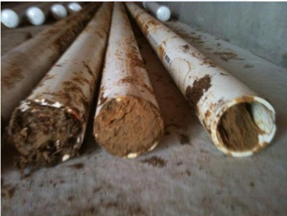
*Figure 6. High fat concentrations in slaughter waste can solubilize during composting and flow into the aeration piping!*
