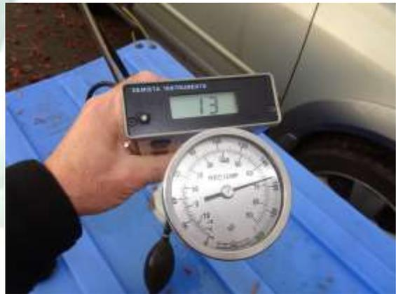
*Figure 3. Measuring temperature and oxygen are important for understanding the success of a compost recipe.*
