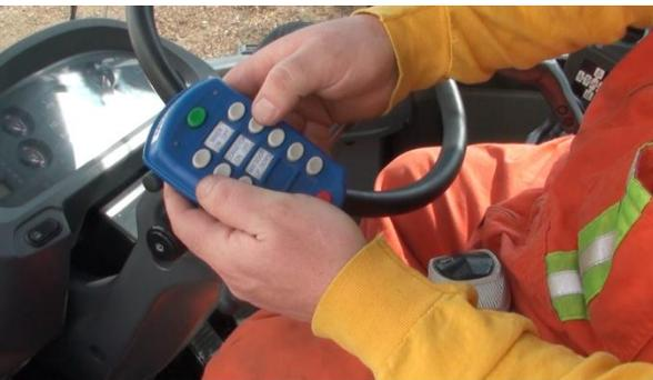
All functions of the mixer are controlled directly from the loader. A status light above the mixer indicates whether the augers are turning, and audible alarms indicate when the mixer and conveyors are being started.
