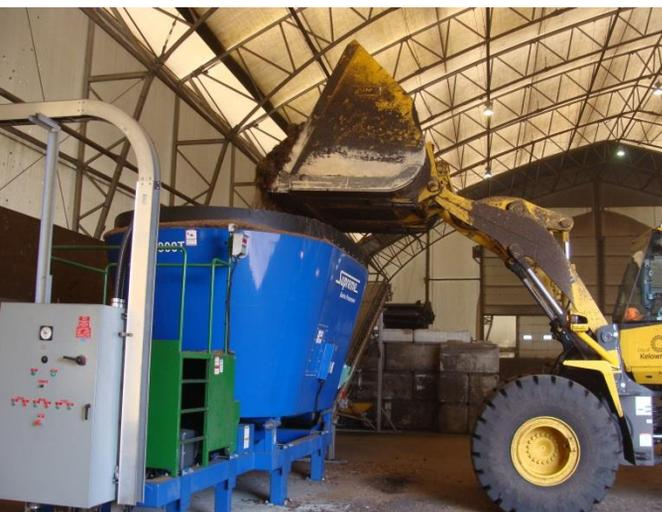
The mix includes two 6 yd buckets of woodchips (approximately 4000 kg) and one 6 yd bucket of biosolids (including some overs, and some ash (approximately 5000 kg), to provide a total batch weight of 9000 kg. The mixing process is less than 2 minutes. The material is discharged from the mixer in less than 2 minutes using a 4 ft wide by 30 ft stainless steel discharge conveyors. The cycle time on one batch for each mixer is 6 minutes. Hourly production is 54 tonnes of blend per hour per mixer.
