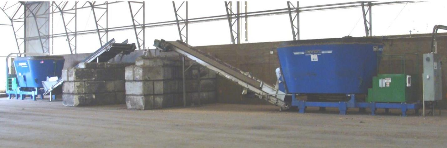
The biosolids composting facility for the City of Kelowna uses two Supreme EnviroProcessor 900 stationary mixers to process up to 54 tonnes of a biosolids compost blend per hour with each mixer. The blended material is then composted on an outdoor aerated pad.
