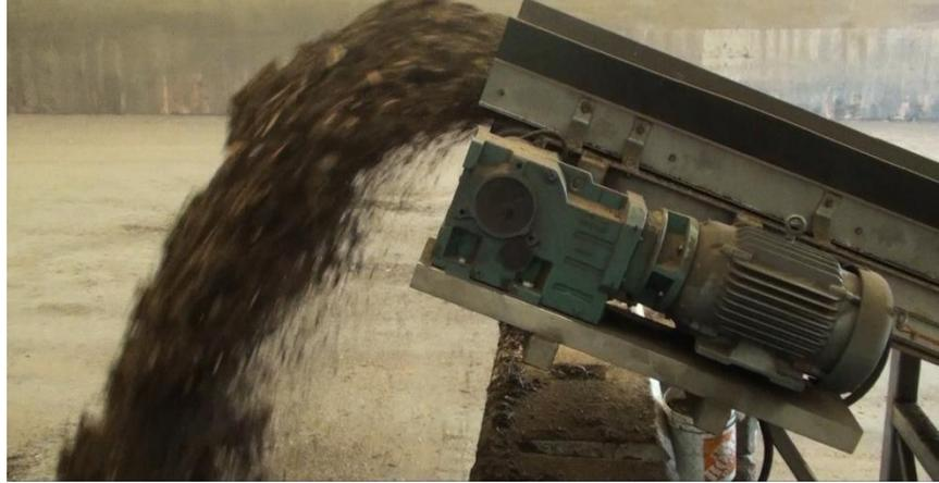
These stationary Supreme EnviroProcessors are powered by 200 hp Baldor severe duty electric motors, which allow them to start fully loaded if necessary. A soft start for the motor and the fluid coupler allow efficient motor starting.
