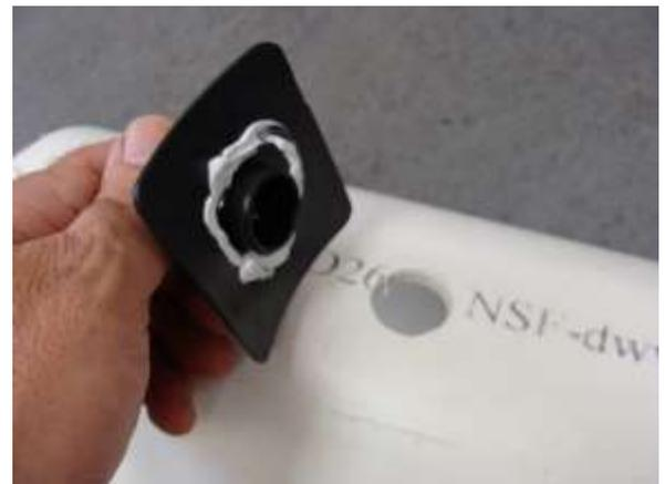
3. Attach the spigot base to the pipe using two screws
