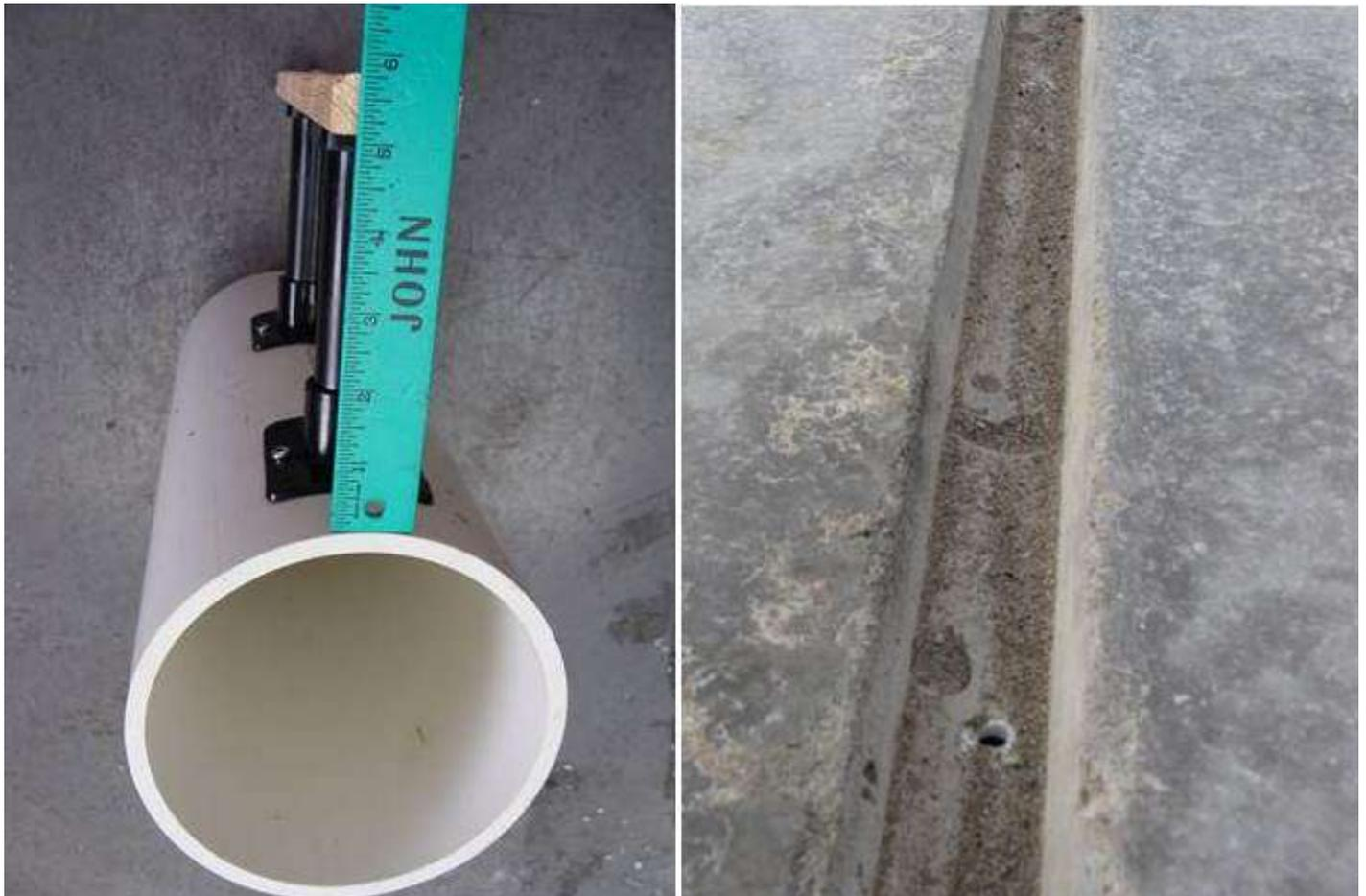
Foundation Air spigots can be easily mounted on 4" (10 cm) or 6" (15 cm) PVC or HDPE pipe. The pipe can be embedded completely in the concrete, or only partially, depending on load requirements. There is no risk of air leakage as the spigots are sealed onto the pipe. The holes are tapered successively
